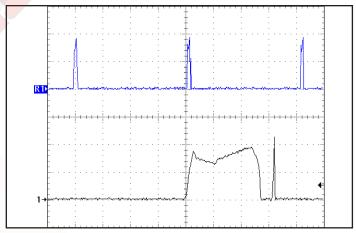
**Figure 18:** Load current (50A/div) as a function of time (2ms/div and 50ms/div) when the converter attempts to turn on into a 10 m $\Omega$  short circuit.
