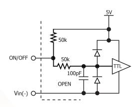
Figure B: Internal ON/OFF pin circuitry
